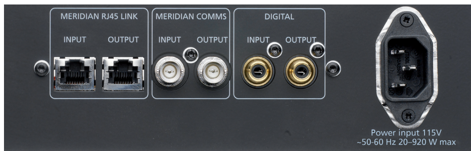
DSP7200 rear panel showing RJ45 connectors.
